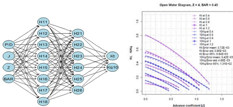
Fig. 6: "ANN analysis and resulting open water diagram for extended propeller series"
