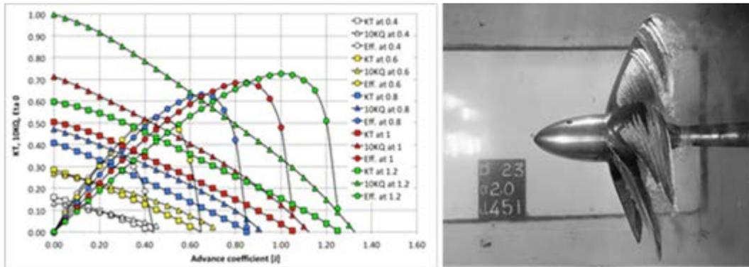
Fig. 5: "Meridian propeller series performance data (KT, 10KQ,  $\eta_p$ ), for varying Pitch / Diameter ratio and cavitation pattern in tunnel test"
