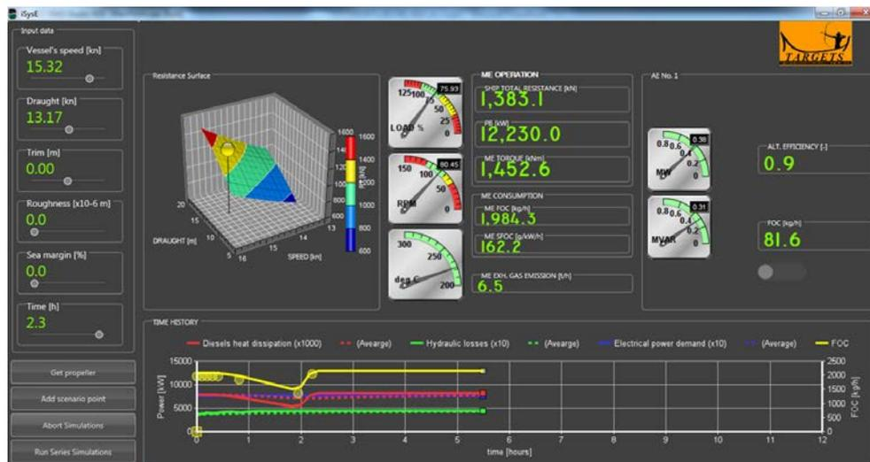
Fig. 13: "DEM Integration: Sample results of simulation in the iSysE application"
