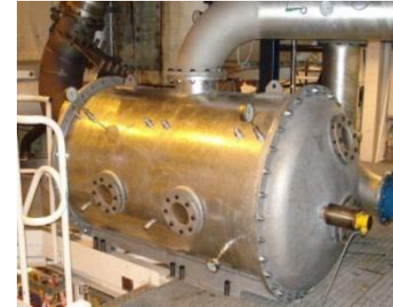
EGR scrubber applied on a MAN 4T50ME-X research engine
