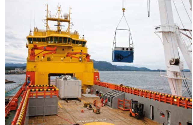
The hybrid propulsion ship mv Viking Lady (with 330 kW MCFC – FellowSHIP)
