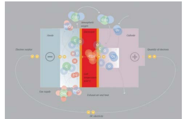
Chemical processes inside a Molten-Carbonate Fuel Cell
